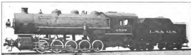
Fig. 21. Ten-Wheel (0-10-0) Switching Locomotive. Built by the American Locomotive Co. for the Lake Shore & Michigan Southern. Cylinders 24 in. x 28 in., Working Steam Pressure 210 lbs. per sq. in., Heating Surface 4,625.4 sq. ft., Diameter of Drivers 52 in., Weight on Drivers 270,000 lbs., Total Weight 270,000 lbs.
